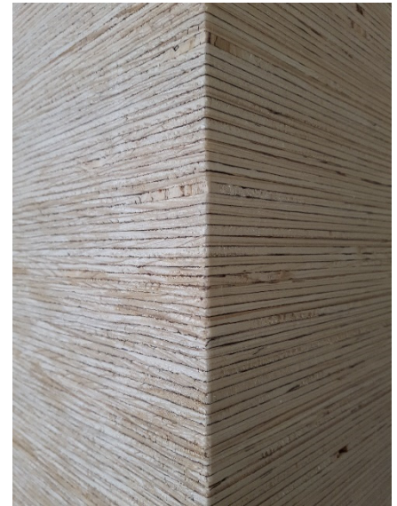
Figure 1. By multiple gluing it is possible to produce even very heavy-duty beams and columns.
