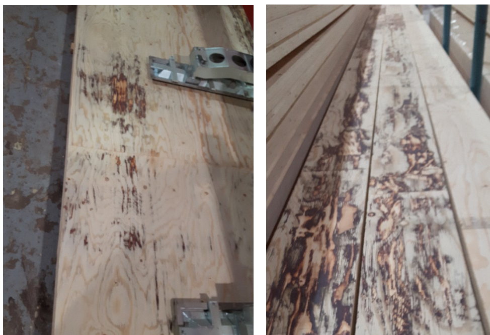
Figure 5. Examples of sanded through face veneers on calibration sanded product.
