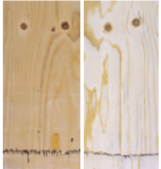
Figure 2. Reverse side, unsanded and sanded, dark brown glue in scarf-joints.
