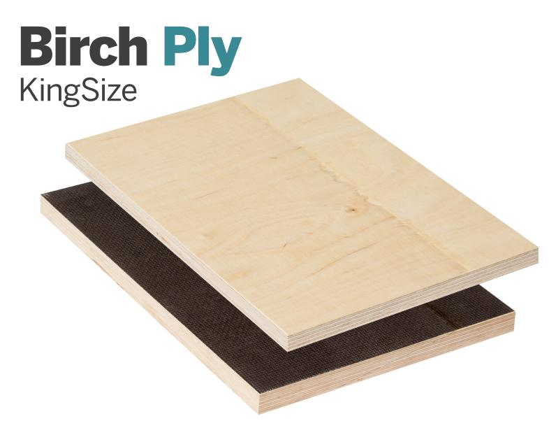
Metsä Wood KingSize is an extra large size birch plywood panel jointed from standard size panels. KingSize panels enable larger one piece components. KingSize panels are available uncoated or overlaid with phenolic film.
