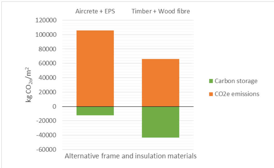
FIGURE 1. Differences in the carbon footprint and carbon storage of the same passive house designed with different frame and insulation materials. Source: Aalto University / Matti Kuittinen.
