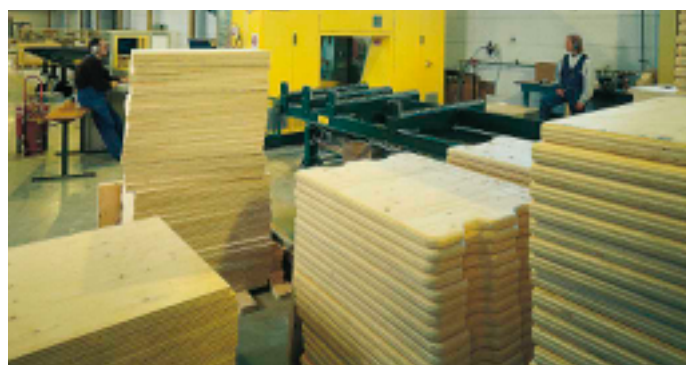
Figure 1. Machined Kerto products in the mill waiting for the packaging and delivery to the customer.
