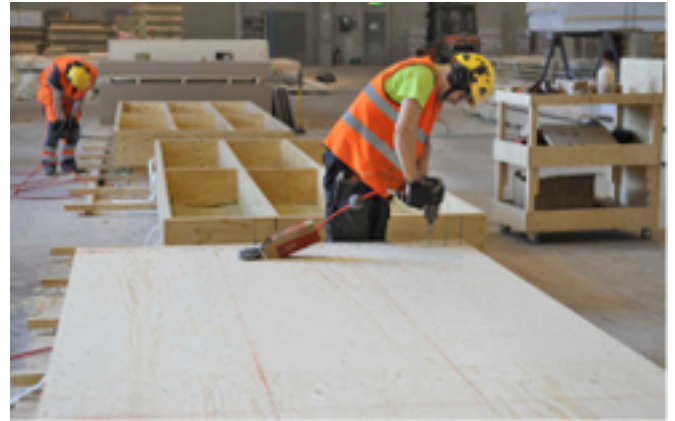
Figure 4. Manufacturing of a Kerto-Ripa box slab.
